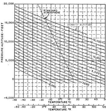
**As summer approaches, temperatures increase and density altitude becomes an important consideration for pilots. High density altitude can affect aircraft in several ways. Wing or rotor lift is decreased. Engine power is reduced. Propeller, rotor, and jet engine**
